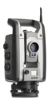
The Trimble® S8 Total Station is Trimble's most advanced total station. Designed to deliver unsurpassed performance in both surveying and specialized engineering applications, the Trimble S8 offers 1" angular accuracy and EDM precision of 1 mm + 1 ppm, plus numerous features to enhance efficiency and productivity.
