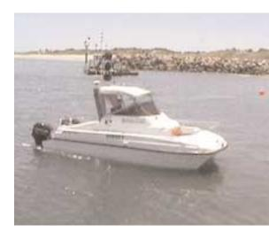
both man-packs and 4WD mounted systems. When not in use onshore the RTK systems are used on the survey boat to provide real-time tide and heave corrections.
