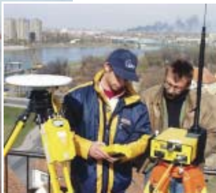
Dj.Ninkov and C. Krulj use the Trimble 5700 GPS Base Station and TRIMTALK 450S UHF radio modem for RTK measurements.
