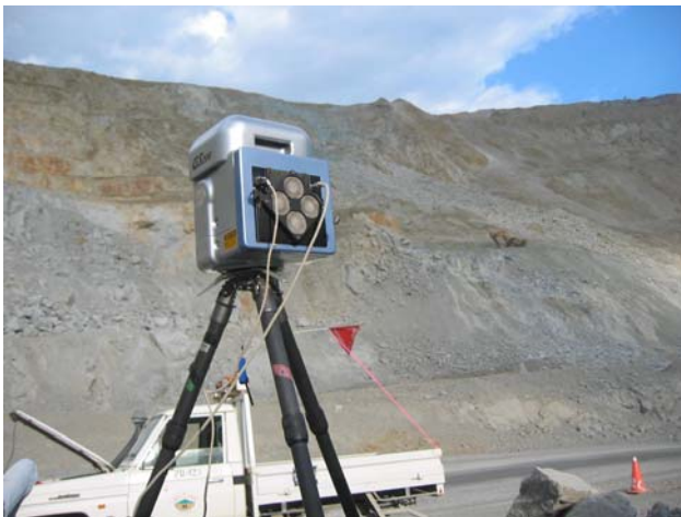
Fig. 9: Pit wall surveyed with Trimble GS-Series
