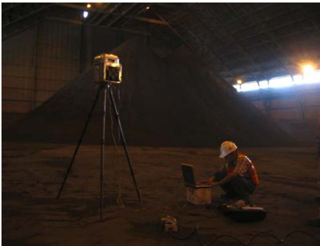
Fig. 6: Stockpile surveyed with Trimble GS-Series.
