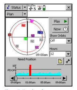
Figure 5: User interface on a professional receiver showing satellites (above) and PDOP (below).
