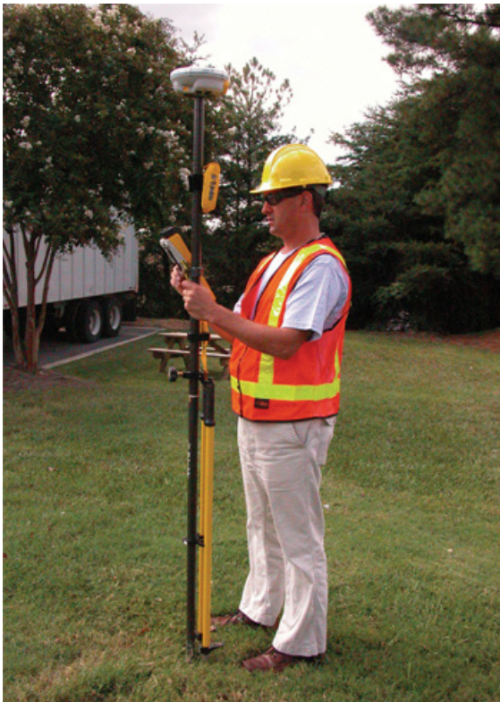
Travis Pruitt and Associates surveyor Patrick Carey uses the Trimble 5800 RTK GPS survey system to locate features for an ALTA survey within the eGPS Trimble VRS network area.
