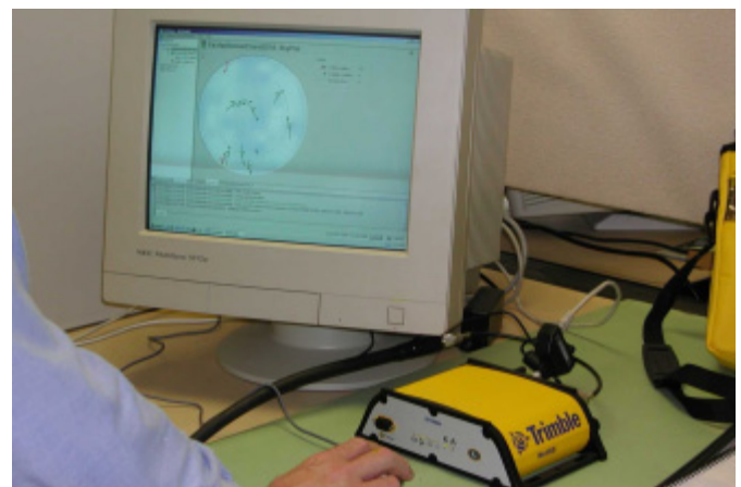
A Trimble NetRS GPS Receiver operating with GPSBase™ software in BC Consultants office.
