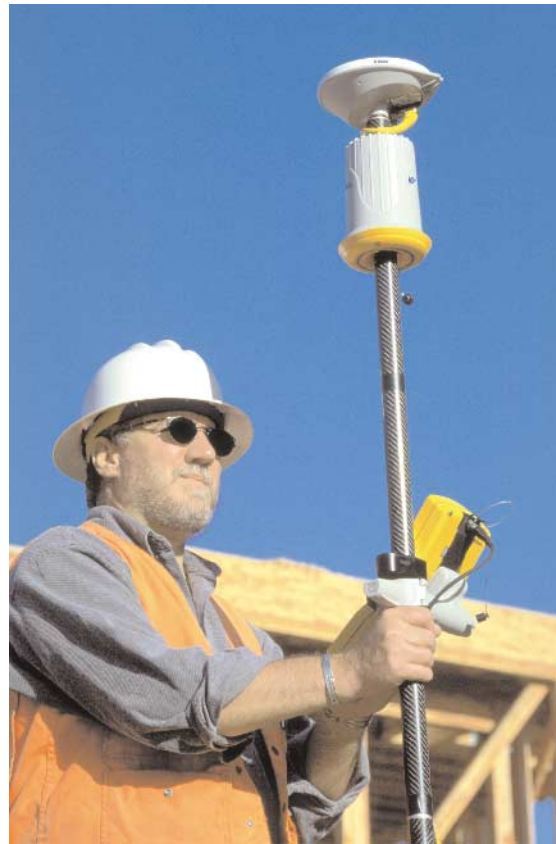
Figure 5. The Range Pole Antenna
