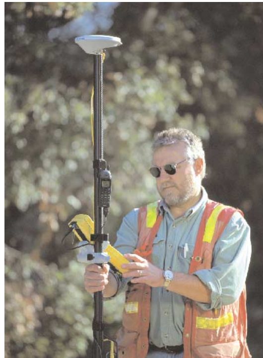
Figure 7. A Cellphone Used with eRTK
